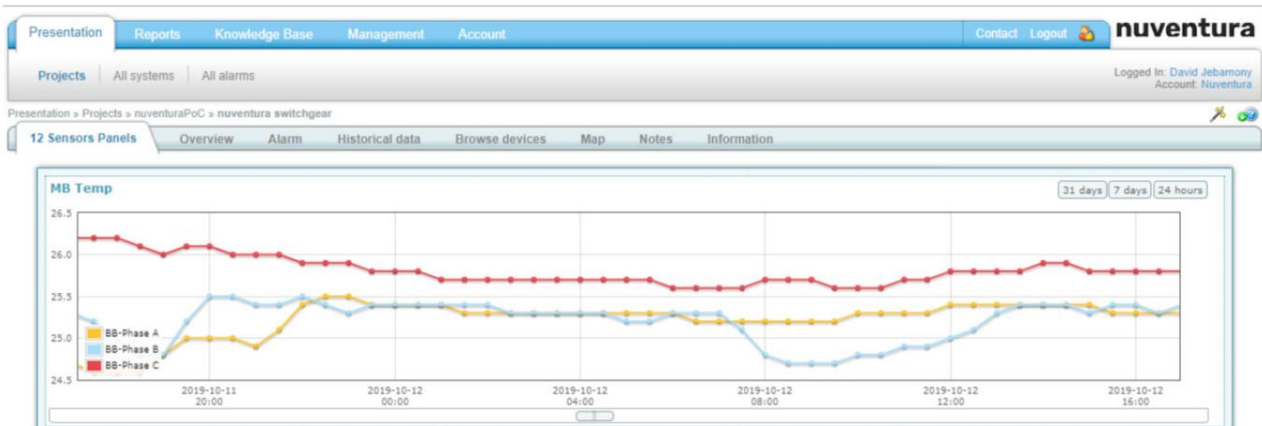
Customizable dashboard with real-time graphing of temperature across different phases
